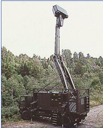
The "Giraffe", Air-warning Radar Unit
