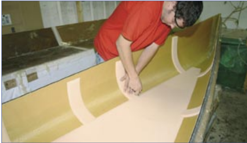
The Divinycell ribs being fitted into a We-no-nah ultra-light canoe.
