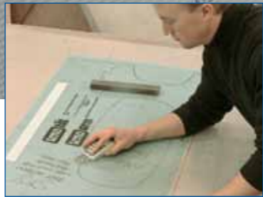
Digitizing mold templates.
