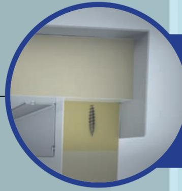
To achieve the desired overall structural integrity of the box, the assembly of the corners is very important. High density structural core is used in combination with aluminum profiles to strengthen the most stressed areas. The assembly is simplified through the use of screws into the structural core for fixation while bonding. The structural core is insensitive to rot or decay and provides consistent screw retention properties.
